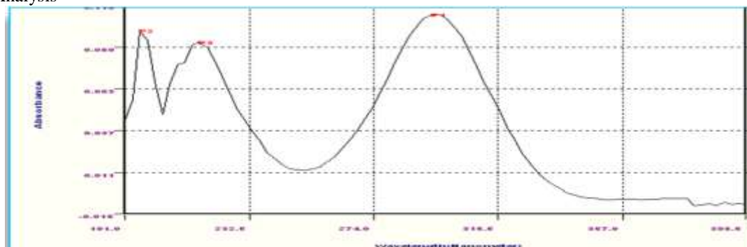
Fig 1: Absorption maxima of timolol maleate
